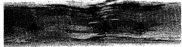
Figure 9 Tensile surface of an anomalously low-strength specimen showing poor fibre alignment.
